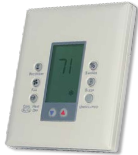
The SS5000 Energy Management Thermostat is a digital computerized intelligent thermostat that controls HVAC systems with a common thermostat interface.
